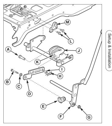
Figure 4. Lift Components - Tilling
